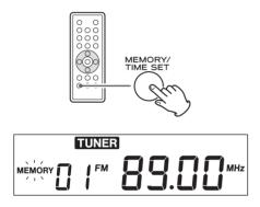
Within 5 seconds, select a preset channel to store the station using the PRESET buttons.
